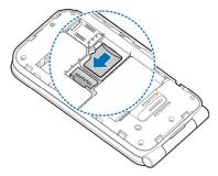
4. Insert the battery, making sure the connectors align. Gently push down on the battery until it clicks into place.
