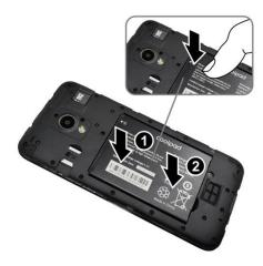
• Align the contacts of the battery with the contacts in the phone.
